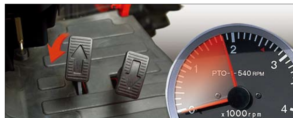
HST Linked pedal(HST) When the HST linked button is engaged, the HST pedal and the engine rpm become synchronized.This greatly simplfys tractor operation and reduces fuel consumption.
